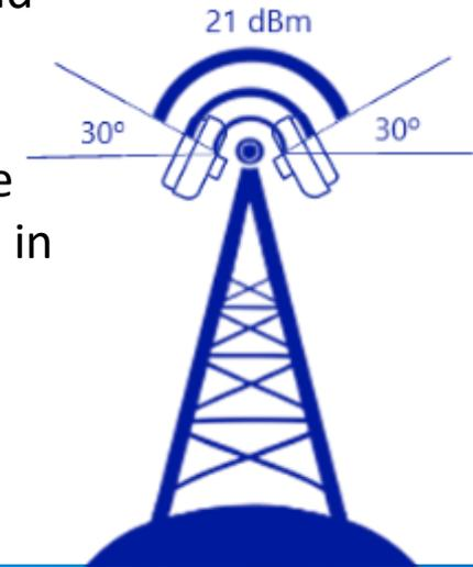
EIRP for outdoor Standard Power device must be **below 125 mW (21 dBm)** for antenna elevation **greater than 30°** above horizon.
