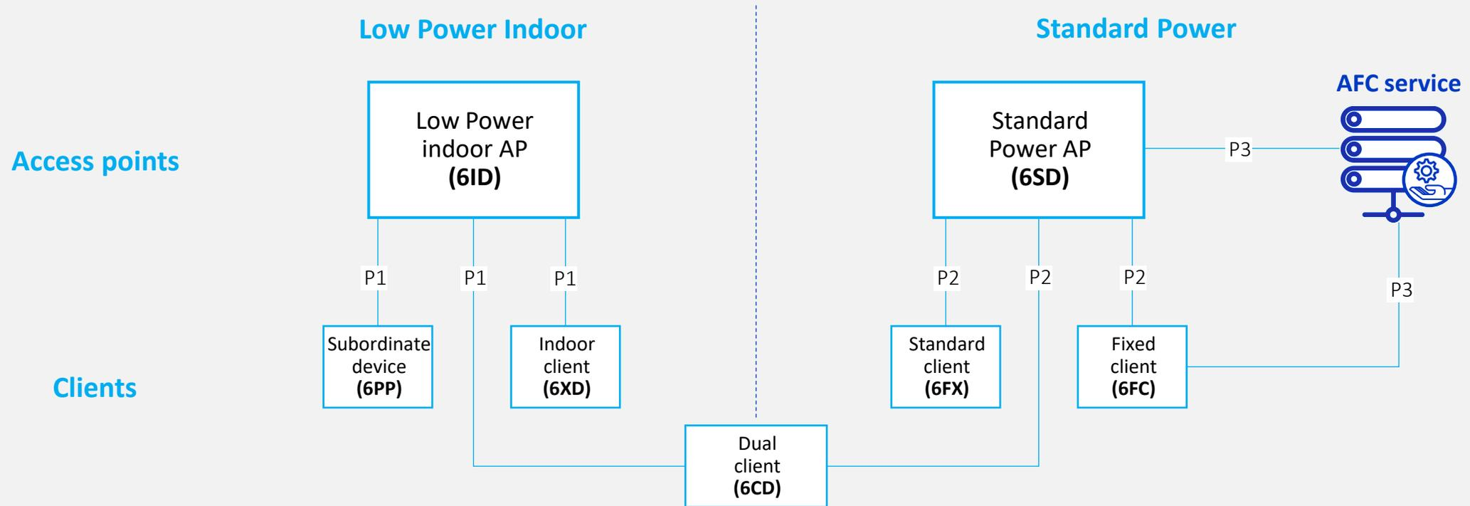
P1: Client and subordinate devices under control of Low Power indoor access point.
