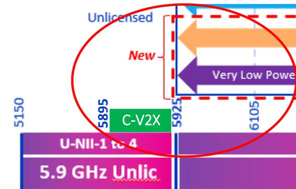
Must prioritize spectrum above 6105 MHz to ensure that C-V2X safety of life services below the U-NII-5 band are protected from harmful interference.
