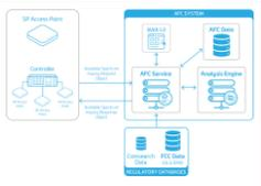
AFC is the 3<sup>rd</sup> generation of centralized DSM methods
