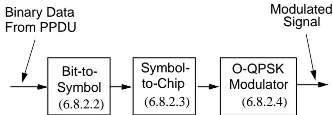
Figure 24—Modulation and spreading functions
