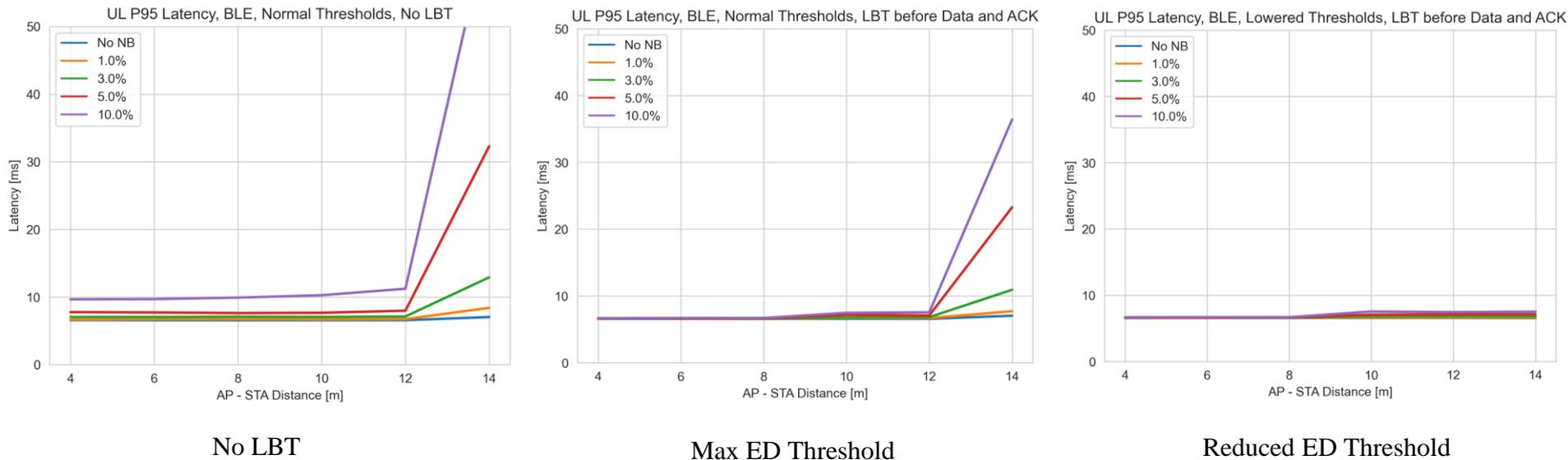
At 14m, AP does not defer to NB C or P nodes, since NB power < -62 dBm
