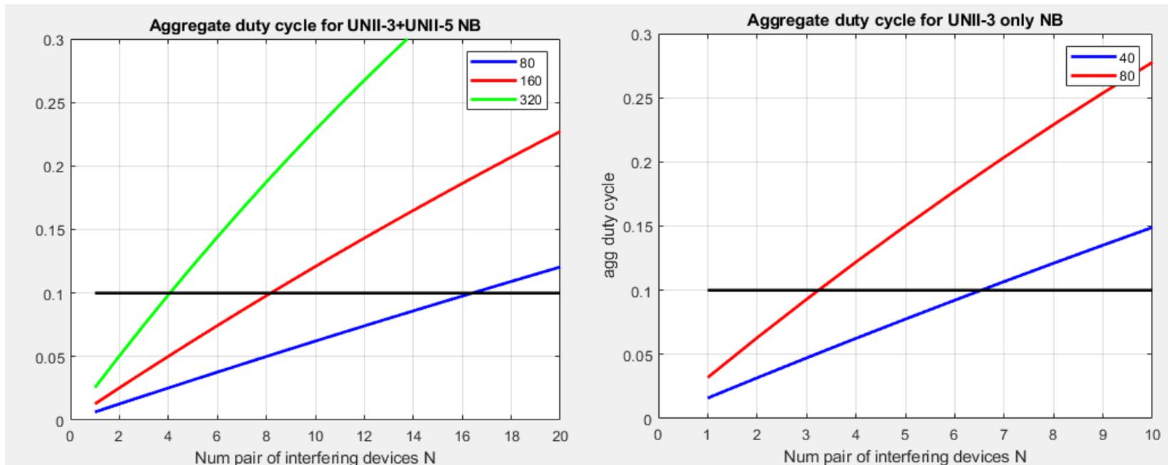
We can reach ~10% aggregate duty cycle with x=5% duty cycle with 4/8/16 (UNII-3 + UNII-5) NB pair of interfering devices on a single 320/160/80 MHz 802.11 channel.
