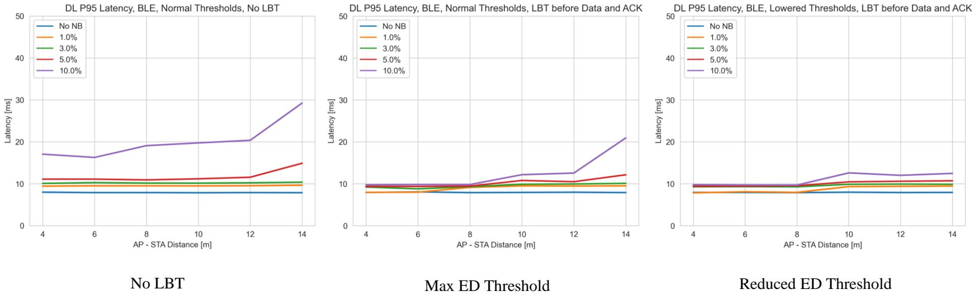
For No-LBT, P95 latency for 10% duty cycle is ~3.6x no NB case
