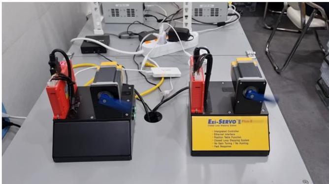
If you continuously send control signals to both motors at 30ms intervals and stop the motor after a certain period of time, you can see that both motors stop at different positions.
