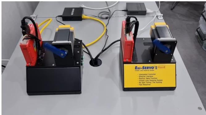
If you continuously send control signals to both motors at 30ms intervals and stop the motor after a certain period of time, you can see that both motors stop at the same position
