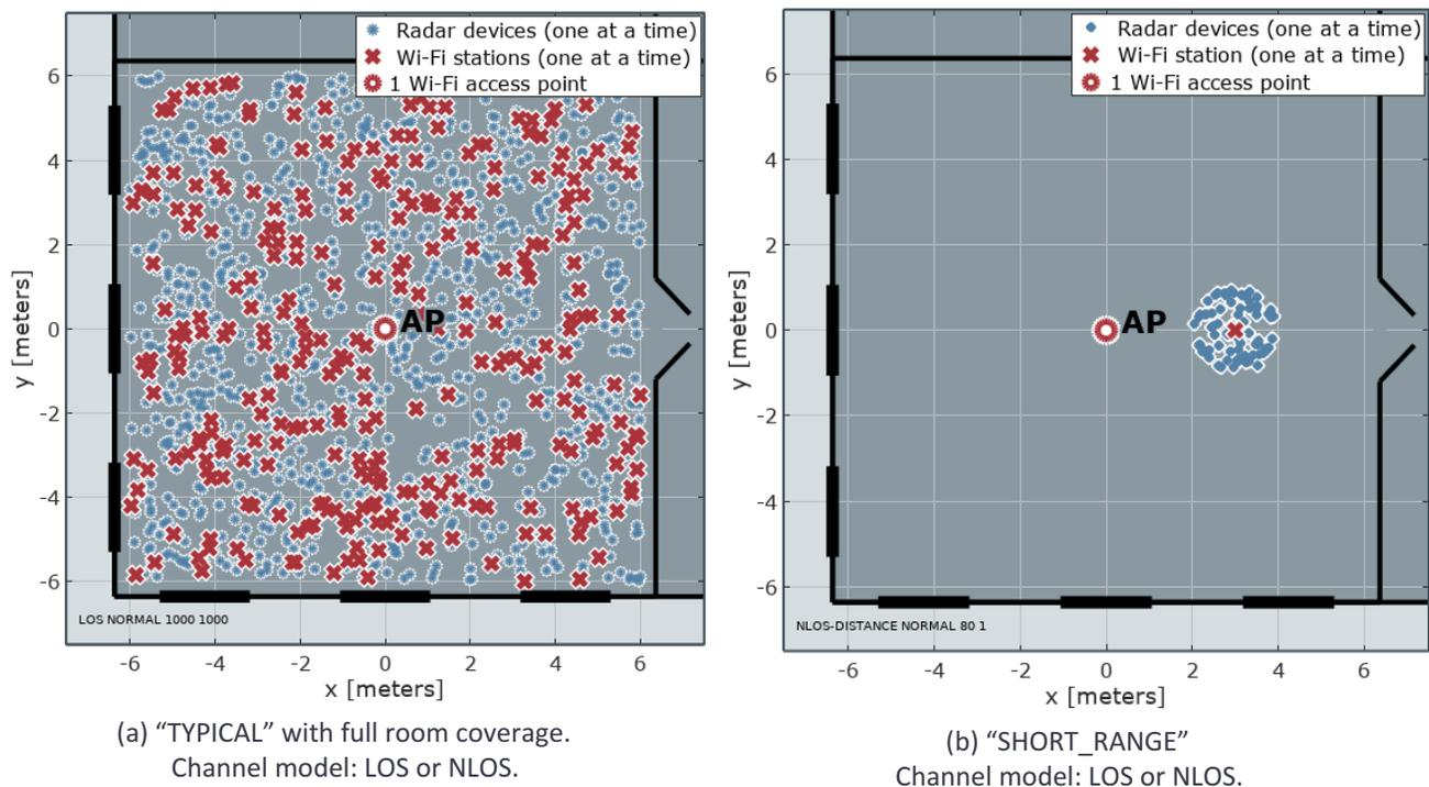
**Figure 12: Simulation scenarios.** There are always only three devices in each simulation experiment: One Wi-Fi AP, one Wi-Fi station, and one radar device. The Wi-Fi antennas always point to each other. The radar antenna always points to a randomly selected direction and therefore the radar's main beam may or may not hit the main beam of the Wi-Fi receiver.
