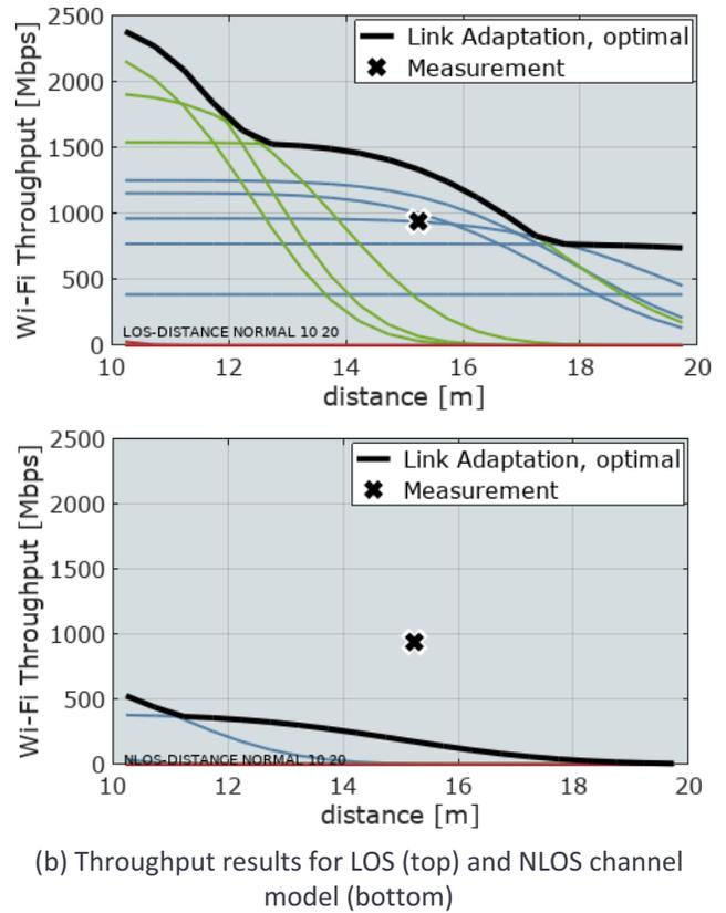
Figure 17: Downlink measurement scenario (a, left), and throughput results for LOS and NLOS (right).
