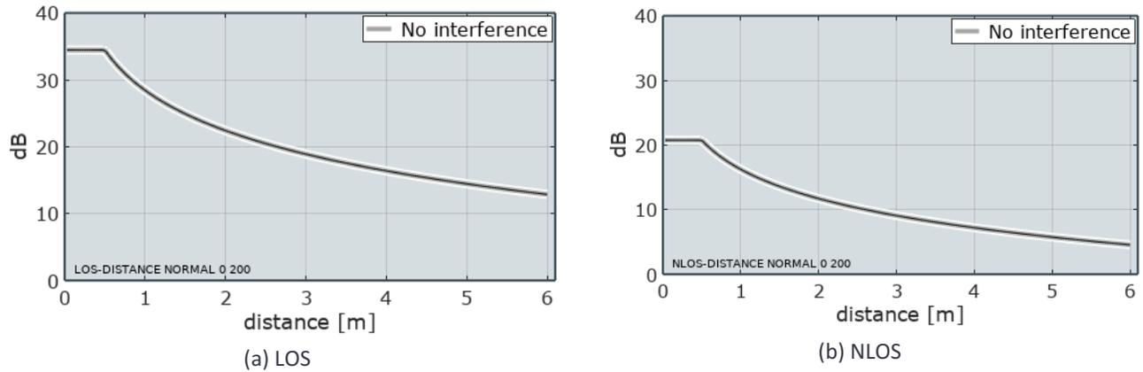
Figure 1: Signal to noise ( $E_{av}/N_0$ ) ratio over distance between radio devices (Wi-Fi or radar) for two channel models. The effect of the reference distance (0.5 m) and the influence of parameter A in both models can be observed.
