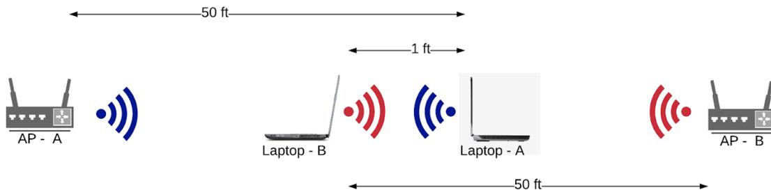
During the measurement, Laptop-B was placed in two positions with respect to Laptop-A as shown below.
