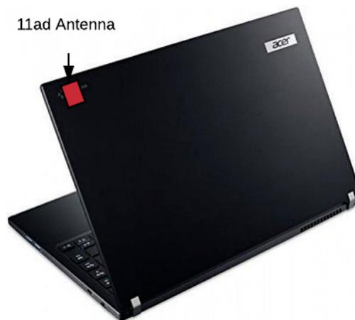
The Soli technology was positioned in various configurations with respect to the 802.11ad antenna, and at various distances for each configuration. The different locations are shown in the figures below. As noted above, the purpose of this study is to examine close-range interference. Accordingly, distances between one inch and one foot were tested. In order to test
