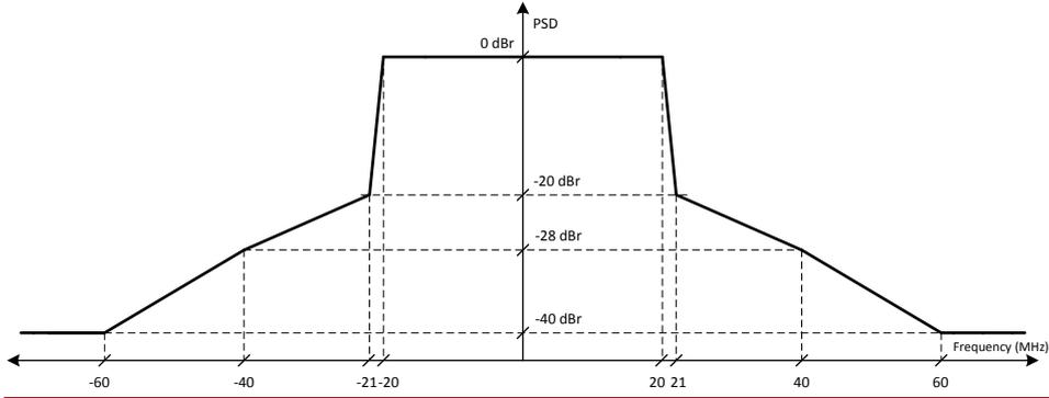
NOTE – The spectrum emission mask is defined relative to the maximum power density in a 1 MHz measurement bandwidth within the channel bandwidth. The relative power of any transmitter emission shall not exceed the levels indicated by the mask or -30 dBm/MHz whichever is the greatest.
