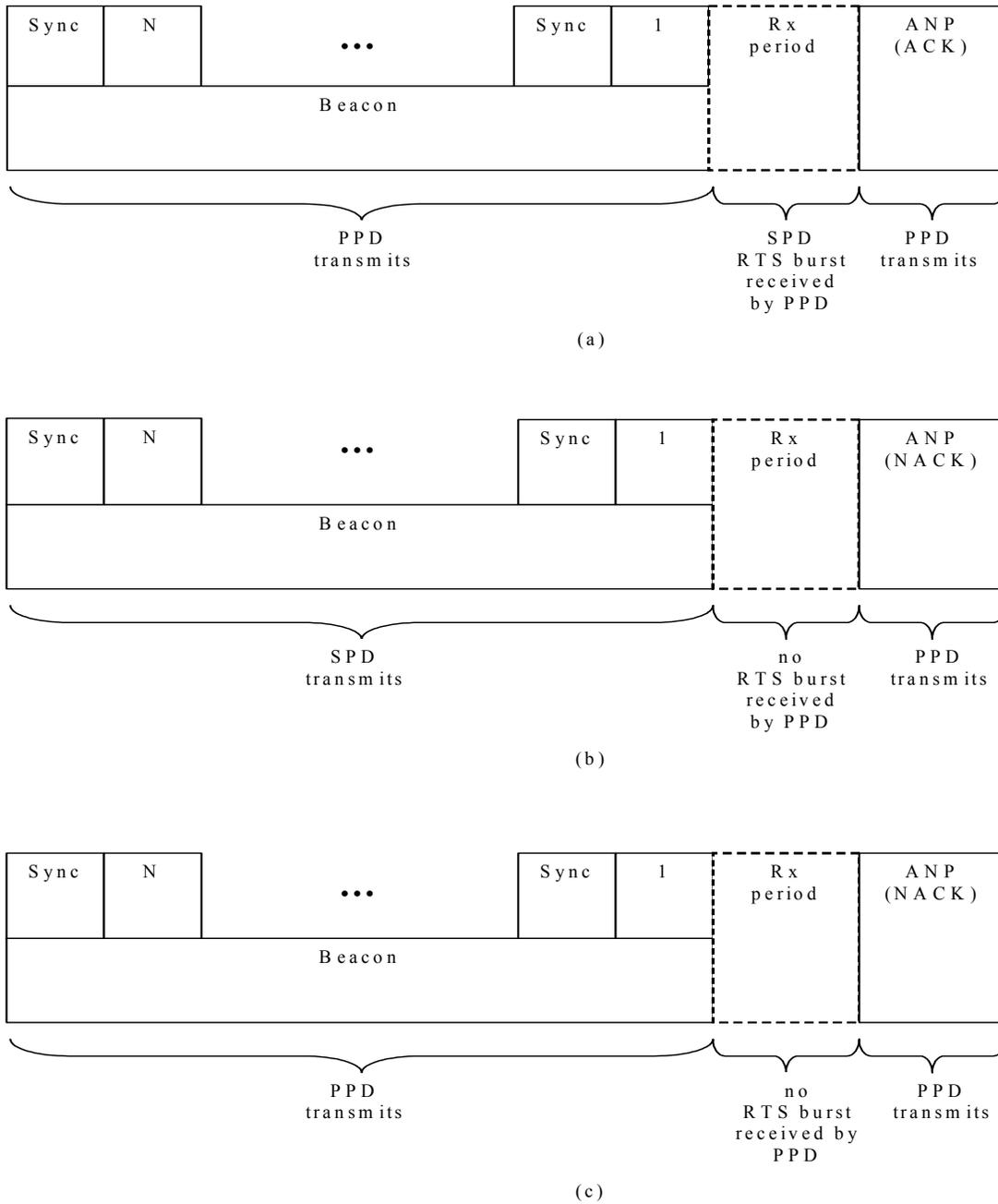
Figure 18—SPD interruption of the PPD in order to transmit a beacon frame
