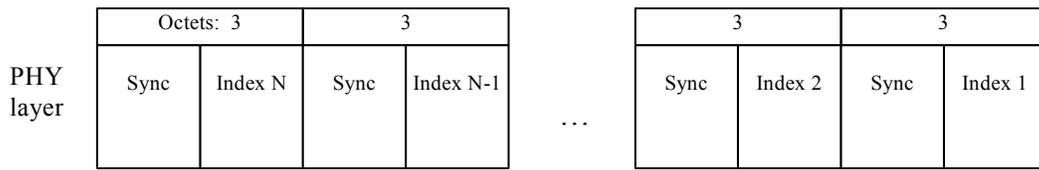
**Figure 4—Schematic view of synchronization burst sequence**
