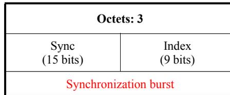
**Figure 7—Format of the PPDU**
