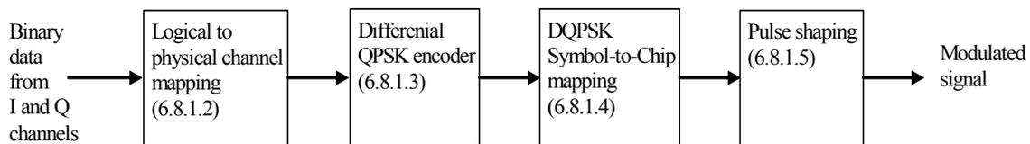
**Figure 9—Modulation and spreading functions**
