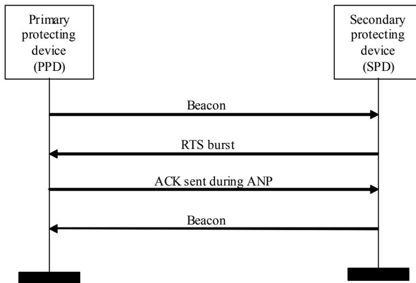
Figure 3—Communication from secondary to primary protecting devices
