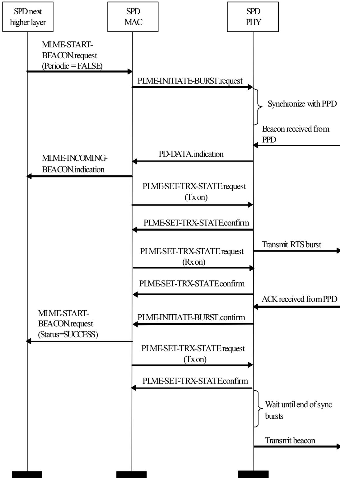
Figure 20—SPD interrupting the PPD (for inter-device communications)
