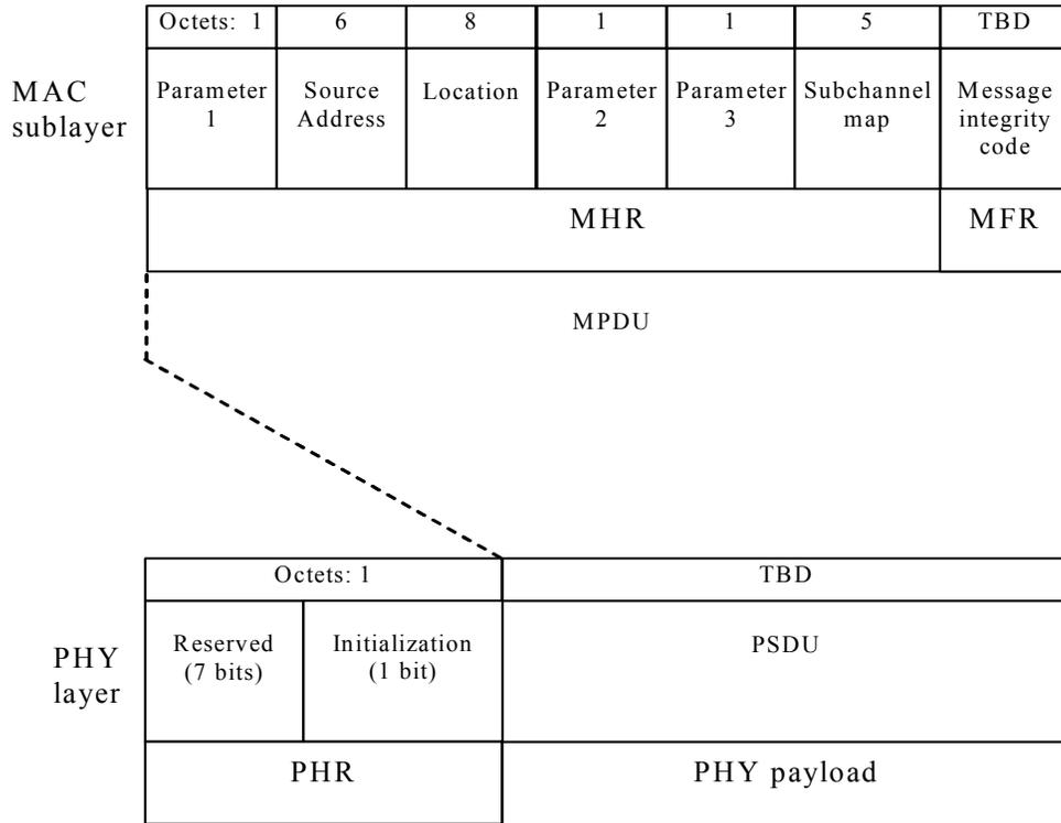
**Figure 5—Schematic view of the beacon frame and the PHY packet (PPDU)**
