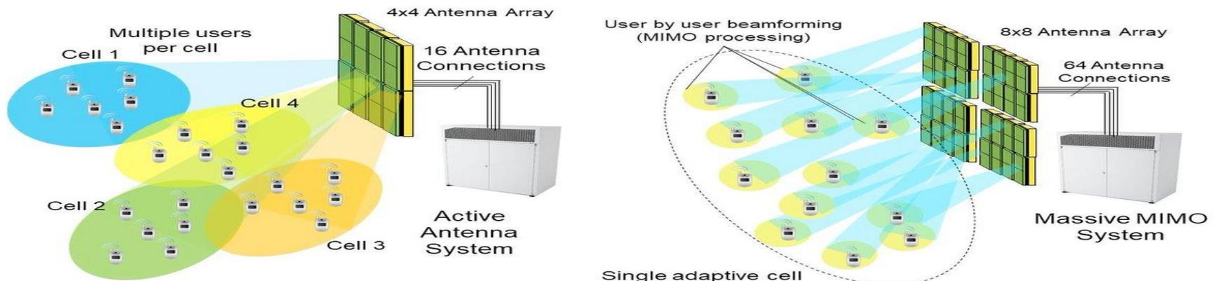
**Spatial Adaptive Beamforming with Massive MIMO is corner-stone of the 5G
