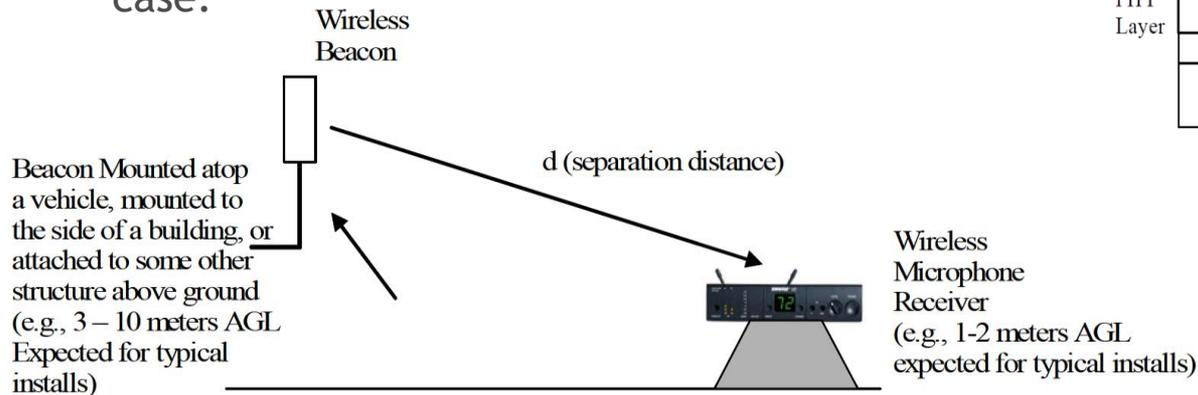
Figure B.1—Beacon/wireless system separation distance
