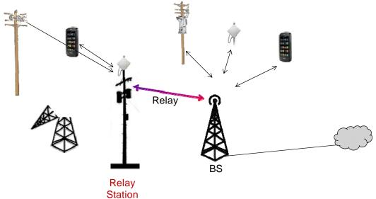
"Mobile" station becomes relay station upon failure of Base Station
