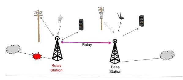
Base Station becomes Relay station upon failure of backhaul
