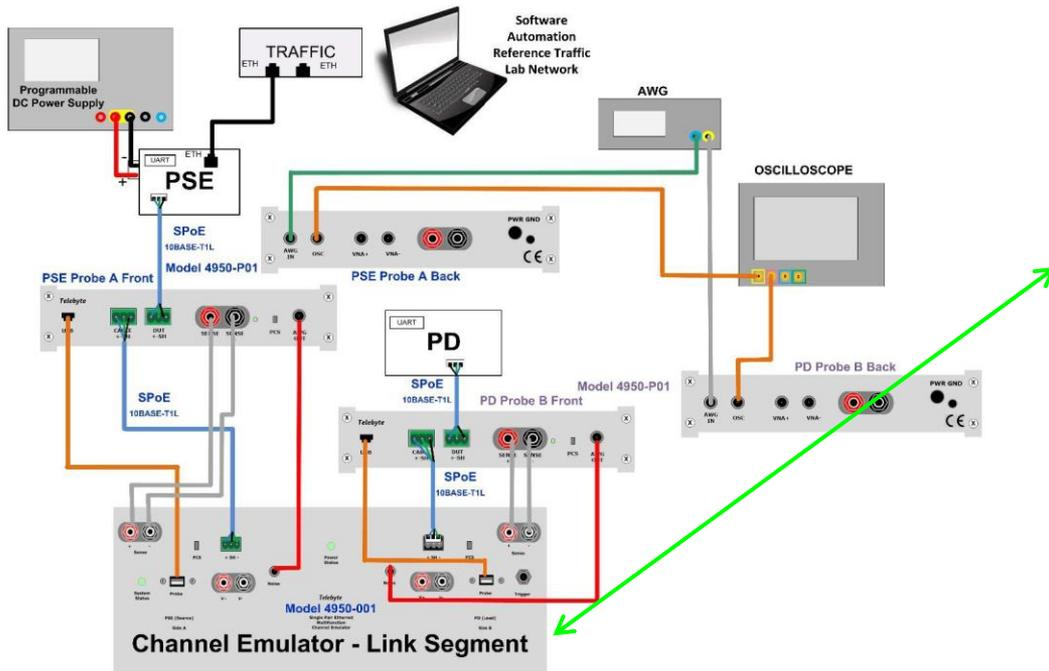
**The Link Segment Channel Emulator** enables the PSE and PD to be tested over different Unshielded Twisted Pair (UTP) or Shielded Twisted Pair (STP) link segments of varying types (Size and Insertion Loss), Delay (Latency), DC Resistance and length.
